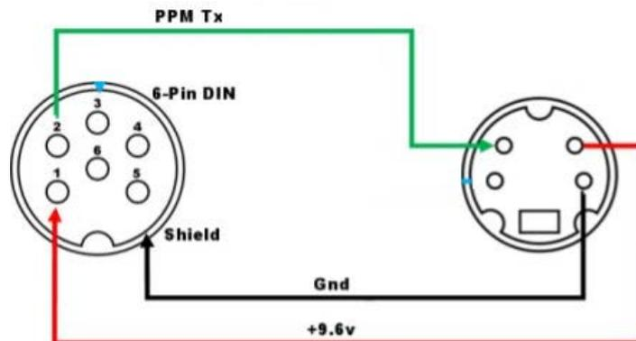
Figure 6. Connection between multiplex DIN connector and EzUHF.
