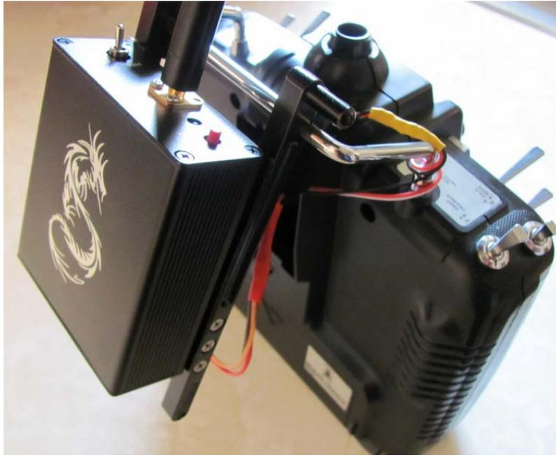
**Figure 2. LRS module installed on a transmitter.**
