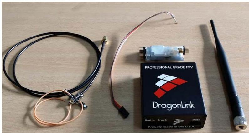
**Figure 3. Elements of a LRS system.**
