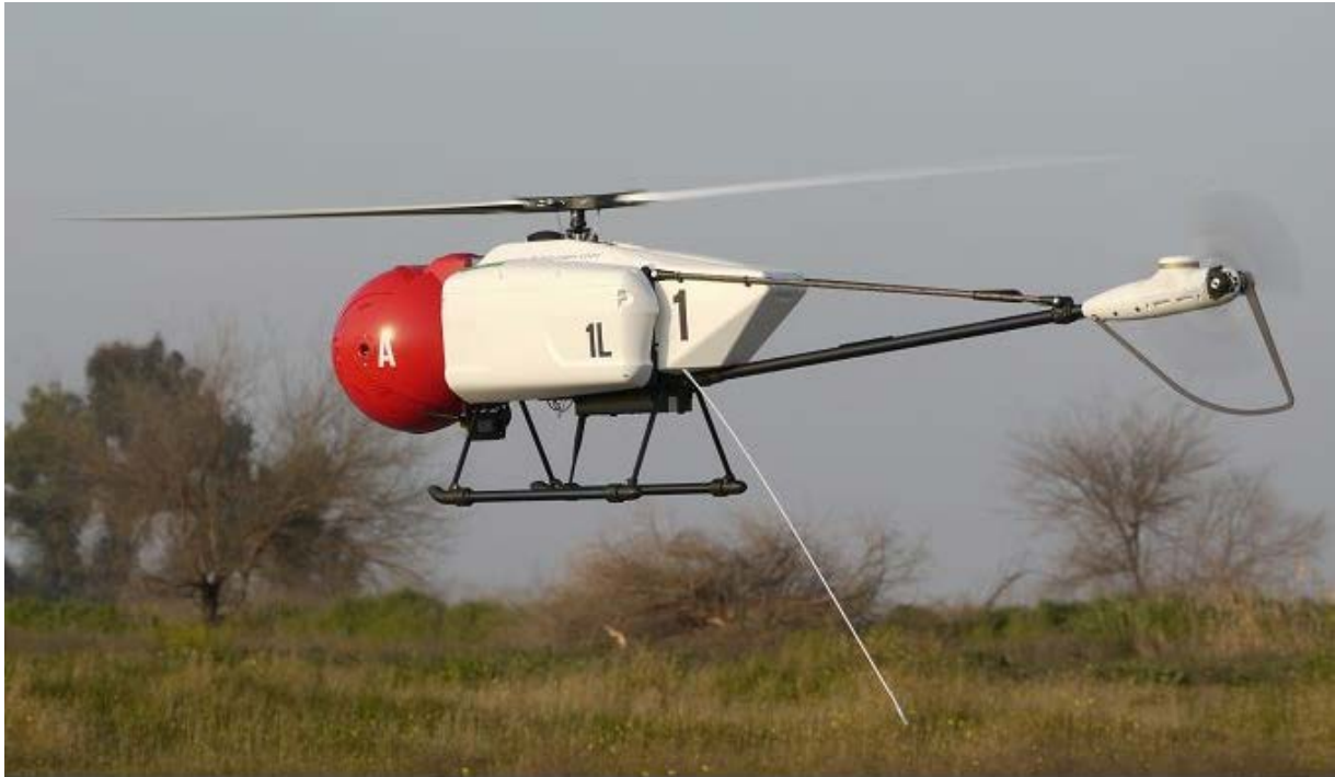
Figure 4. SARAH unmanned helicopters used for the flights. (Photo: CATEC)
